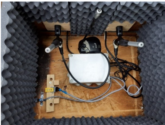
Fig. 1. Picture of the acquisition system installed on a dedicated chamber on top of the beehive.
