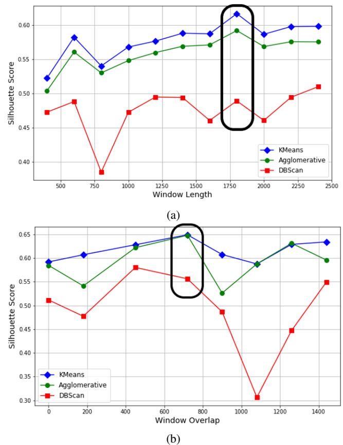
Fig. 3: Impact of the window length (a) and the overlap (b) parameter to the clustering results.
