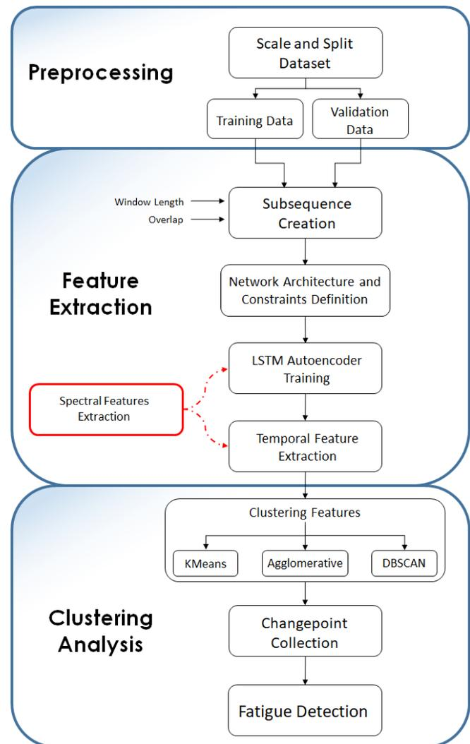
Fig. 1: Algorithmic flow of the training procedure.
