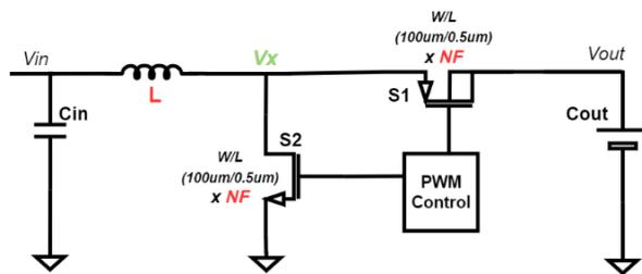
Fig. 1. Boost DC -DC converter schematic
