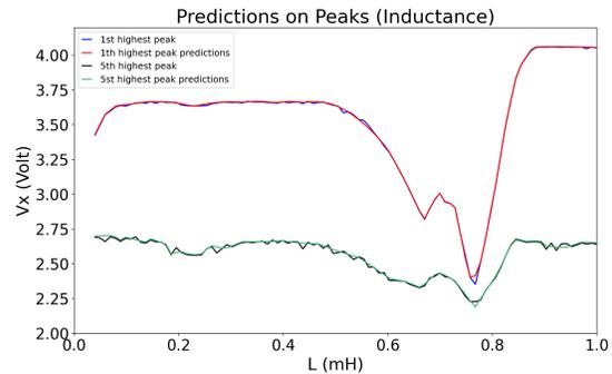
(b)  $V_x$  switch node peak value of the first and fifth highest peaks, with respect to different values of inductance.
