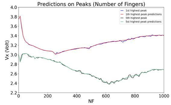
(a)  $V_x$  switch node time domain voltage and model prediction for 1 and 354 fingers (b)  $V_x$  switch node peak value of the first and fifth highest peaks, with respect to different number of fingers.
