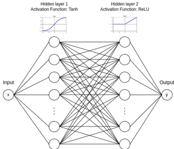
Fig. 3. Architecture of Neural Network.
