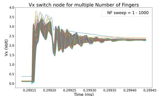
(b) V<sub>x</sub> switch node transient signals for various Number of Fingers.
