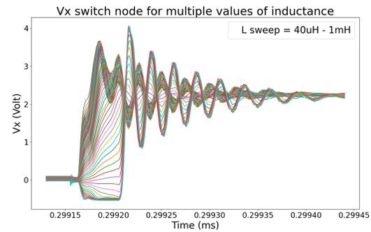
(a) V<sub>x</sub> switch node transient signals for various inductance values
