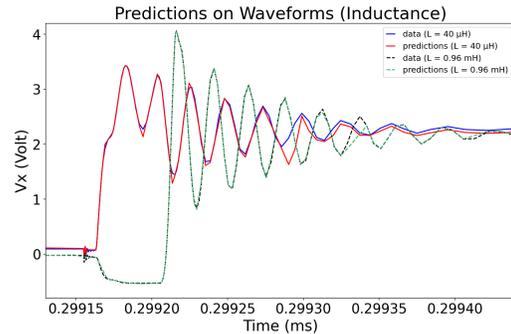
(a)  $V_x$  switch node time domain voltage and model prediction for inductance values of  $40 \mu H$  and  $0.96 mH$
